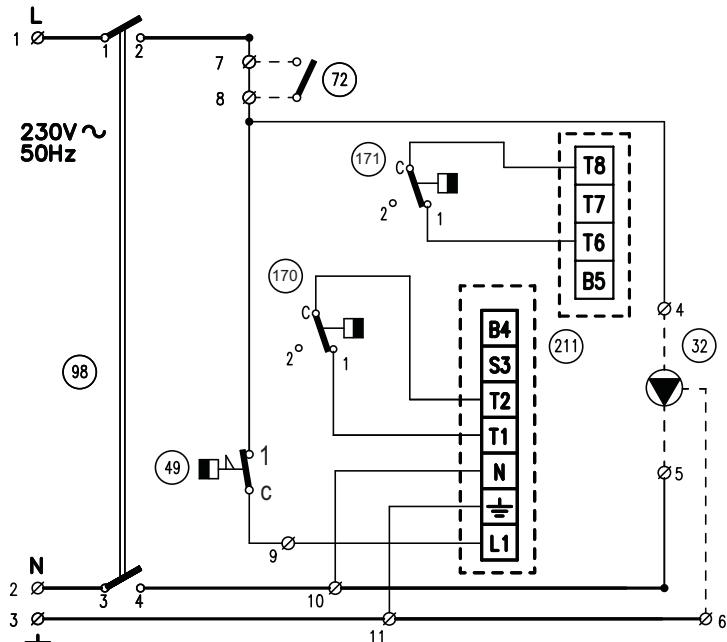
fig. 9 - Main wiring diagram ATLAS 95
