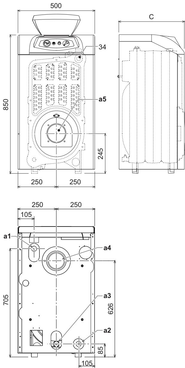
fig. 5 - Dimensions, connections and main components
