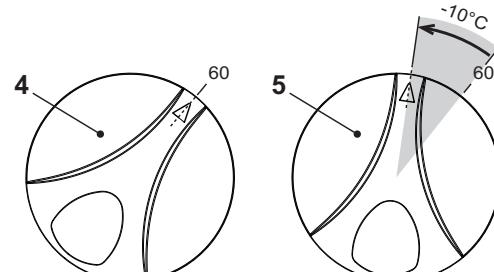
fig. 3 - Temperature adjustment for model ATLAS 95
