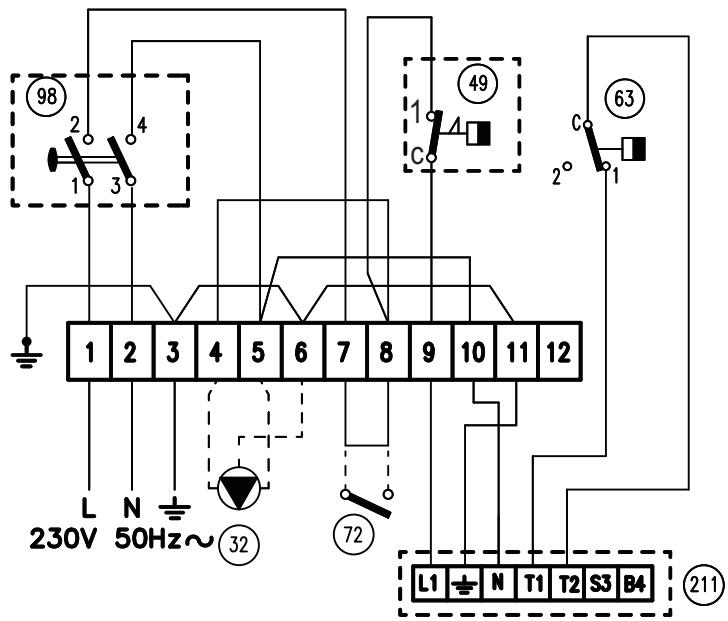
fig. 8 - Electrical connection diagram ATLAS 32-78
