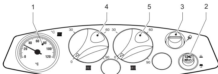
fig. 2 - Control panel for models ATLAS 95
