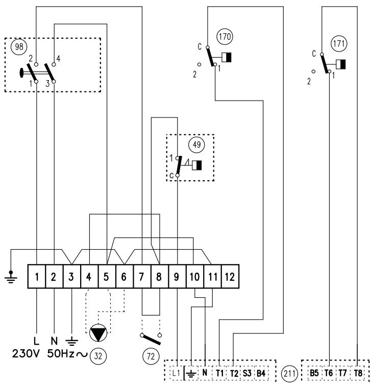
fig. 10 - Electrical connection diagram ATLAS 95
